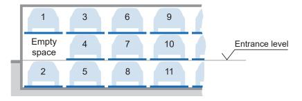
In the default setting the basement platform no. 2 is raised to entrance level (Cover of the pit according to safety regulations).
