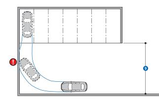
We recommend platform widths of a minimum of 270 cm for edge boxes and boxes with partitions and driving lane widths of 650 cm so that vehicles can comfortably enter and leave the swiss-park-systems without difficulty.
